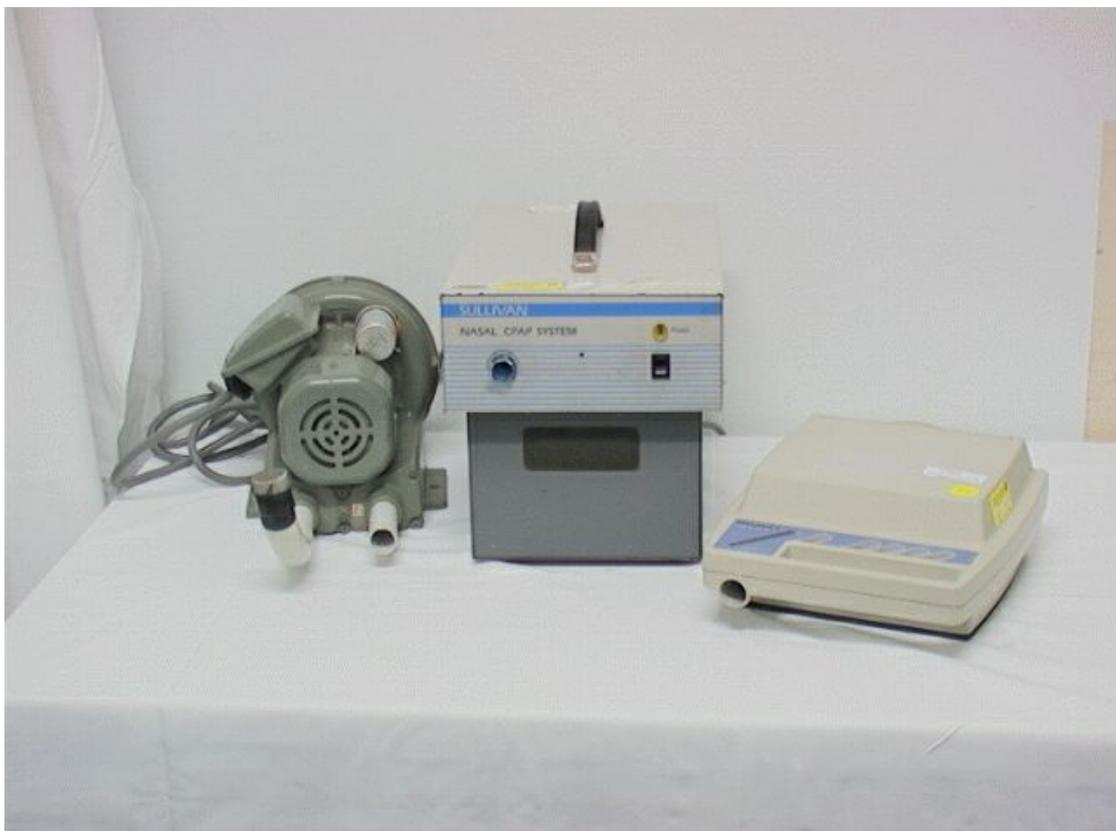
Fig 1 The very first CPAP machine (right) was and off the shelf compressor.
